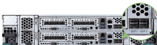
Two 12Gb SAS Expansion Ports per Controller
